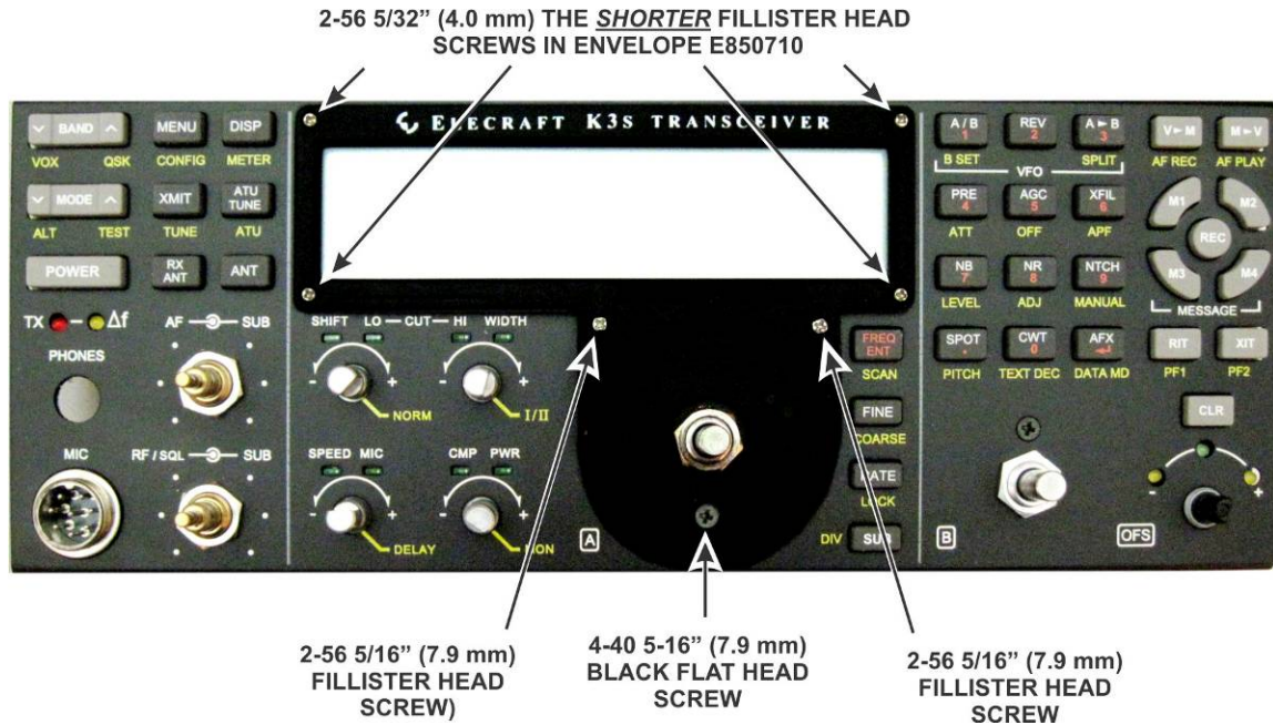
Figure 16. Mounting the Bezel.
