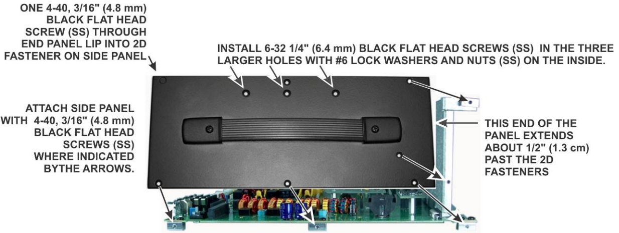
Figure 65. Mounting Left Side Panel.
