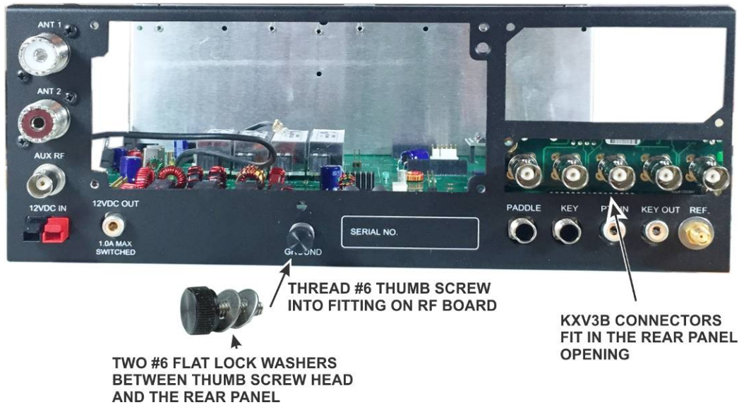
Figure 49. Mounting the Rear Panel.
