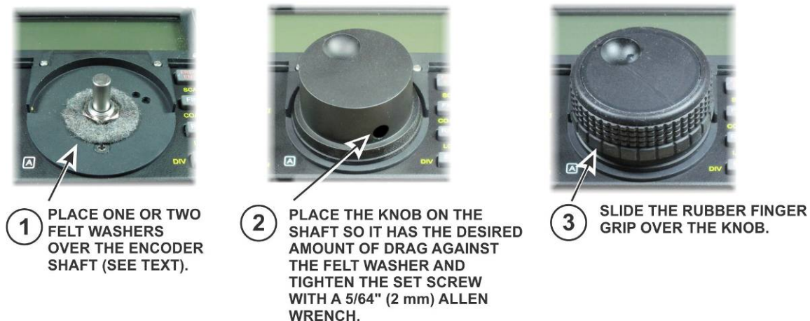
Figure 20. Mounting the VFO A Tuning Knob.
